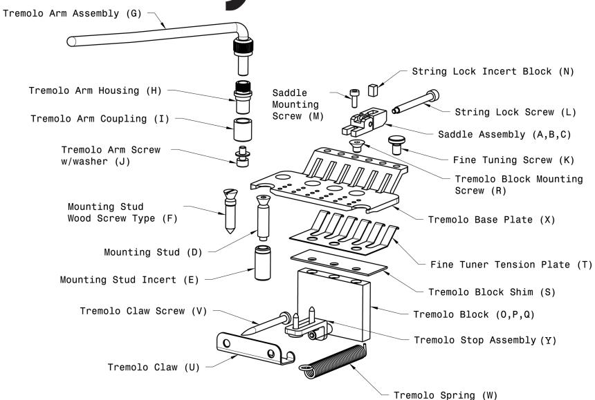
Parts diagram applicable for the following systems: Floyd Rose Original 6 & 7 Strings, 1000 Series Original, Special, and Titanium
