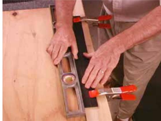
A shooting block is a long, square-edged sanding block for creating smooth, straight surfaces. We used a carpenter's level and fastened the sandpaper to it with double-stick tape (**pictured**).
