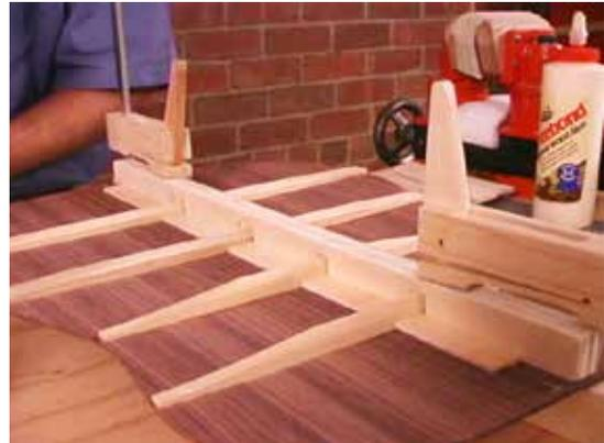
the distance of the spruce center strips. This keeps the reinforcing center strips in a neat, straight line from end to end. Use scrap wood cauls and two cam clamps for uniform pressure on each spruce strip. Avoid glue squeeze-out that might stick to the notched caul!
