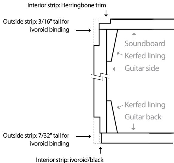
The first pass is for the interior strips and is made with the appropriate bearing on the cutter bit. The router bit should be set to cut a shallow ledge and a width to accommodate both the interior strip and the outside ivoroid binding. Make practice cuts on scrap wood, check the fit of the trim strips before routing the actual channels. Once starting the routing on the guitar body, check the fit before going very far to be sure both the depth and the width are correct.
