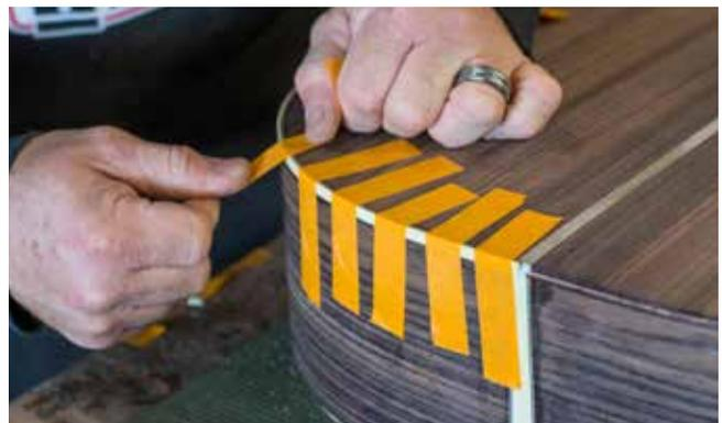
Binding the back: glue the thin ivoroid/black purfling first (ivoroid side in, black faces out) followed by the thick ivoroid binding. The binding joints at the neck block and tailblock must be trimmed for a close fit (**pictured**). Bind-ALL is a solvent based glue, so it will melt the joints together. Allow 6-8 hours drying time before removing the tape.
