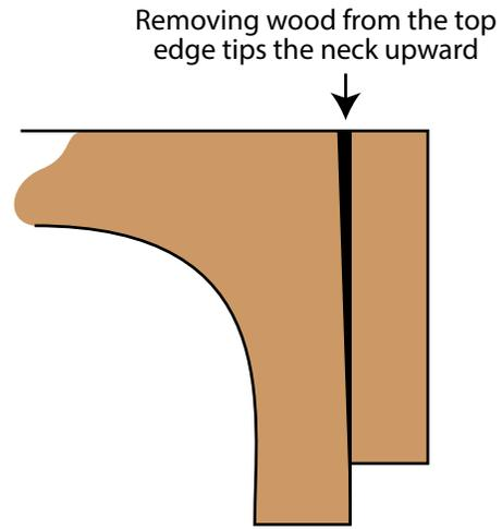
cheek. Cut in the direction of the top edges. A final light, downward pull of the sandpaper strip will clean up any marks left by the chisel.
