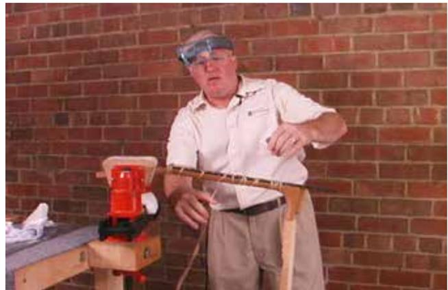
the neck. Tie the rubber band at the nut end, and start wrapping **(pictured)**. The fretboard will align itself as you wrap, and can be easily moved if one edge is off-center. Stretch the rubber band tightly as you wrap toward the neck heel, go around the neck joint and the heel, and then wrap back to the nut. Even with a light glue application, you'll probably get a lot of glue squeeze-out. Wipe off excess glue and let the neck dry overnight.
