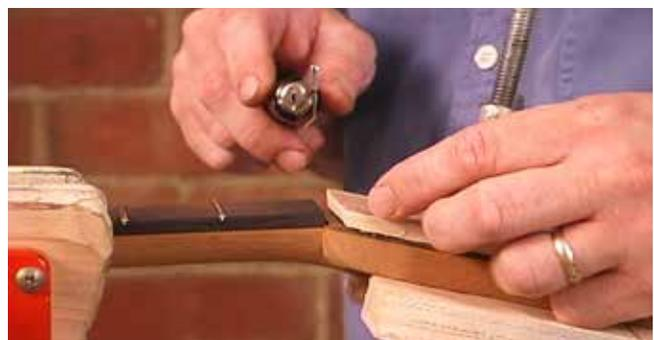
Lightly glue the nut in place with a couple of drops of Titebond in the mahogany slot, and a couple of drops on the end of the fretboard. You can sand the edges of the nut when you final-sand the neck.
