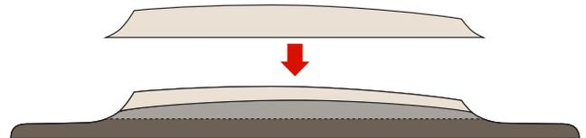
bridge and you want to achieve a smooth transition where the bone and wood meet. Switching to higher and higher grits of sand paper as you get closer to the final shape helps with this process. When the fit is perfect hand polishing the bridge and ends of the saddle with micromesh will give the bridge a nice shine and smooth feel.
