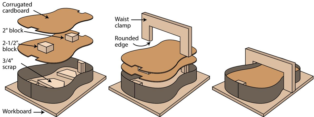
Next, glue a 2" thick block of scrap wood onto the cardboard, centered about 4" from the smaller end of the guitar mold. Then glue a second 2-1/2" piece of scrap wood, centered about 4" from the bottom (larger end) of the guitar mold. Glue the second piece of cardboard onto them. Now the two cardboard forms are fastened together with blocks of wood between them, creating a three-dimensional form for supporting the guitar sides.
