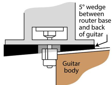
Double stick tape the  $5^\circ$  wedge to the bottom of your router base. You'll use this wedge for routing from the neck block area all the way to the last brace in the lower bout. Once you get to the last brace, remove the wedge, read just the height of the bit, and finish the cut to the center of the tailblock before stopping again. This will be repeated on the opposite side of the body.
