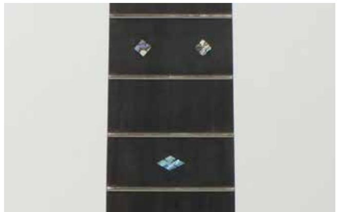
Use just a touch of super glue or black epoxy to permanently set your inlays. The inlays are a tight fit, so you may need to press them flush to the surface of the fretboard using a hard, flat object. Use wax paper placed between the them—you don't want to have the object glued to your fingerboard if there is any glue squeeze-out. After you press the inlays flush in the center of the fretboard, they will be raised slightly at the edges, since the fretboard is radiused. Use a smooth
