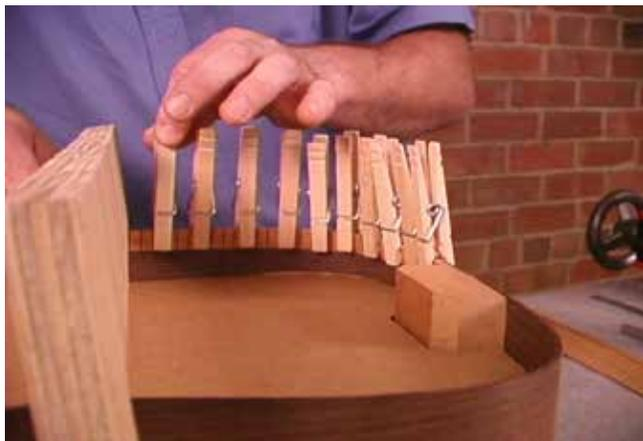
Titebond, check the 1/32" clearance and reclamp. Let the glue dry for 4 hours. Install the lining strips on the back edge of the side assembly in the same manner.
