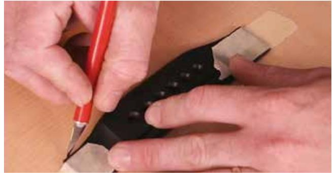
center and sides of the bridge (**pictured**). Use a hand plane, file or sandpaper to match the bridge's contours, and glue sandpaper to the bottom of each caul to help keep it steady when clamped.
