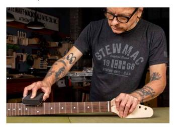
After a complete sanding, wipe down the body and neck with a damp cloth to raise the grain to reveal fibers that need more sanding. Let the wood dry, then sand the raised grain with 220- grit sandpaper. After sanding, raise the grain again and sand a third time, using 320-grit sandpaper.
