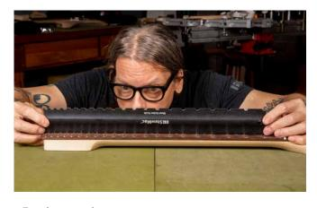
Turn the truss rod nut counterclockwise to bring the neck up, adding relief.
