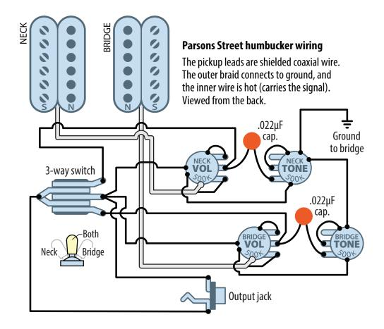
**Modern modification:** In the vintage wiring above, rolling off the tone control slightly reduces your volume. Connecting both capacitors as shown at right fixes this, but you lose a little treble when you lower the volume.
